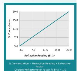
Coolant Refractometer Factor 70 Brix =
